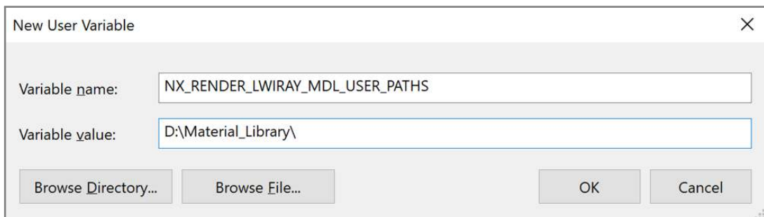
Fig. 3.18 - Defining the value of user variable NX_RENDER_LWIRAY_MDL_USER_PATHS
