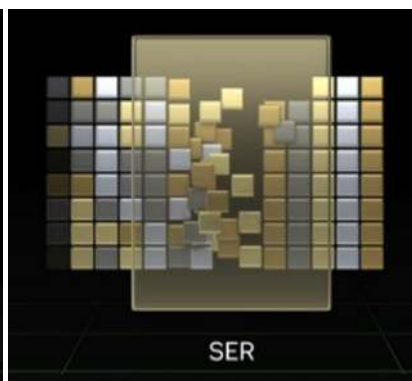
Fig. 8.2 - SER reorders threads, grouping similar work together
