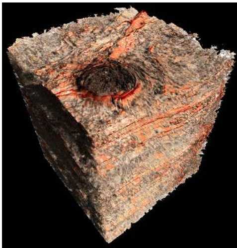
Seismic dataset showing reflectivity and seismic layers using a non-local shading technique (page 11)
