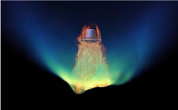
Shows the vorticity field beneath the lander and how it wraps around the vehicle
