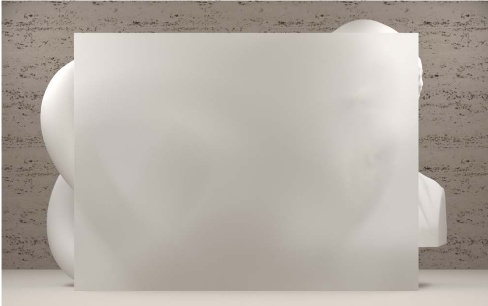
Fig. 3.4 - Diffuse transmission through a thin object
