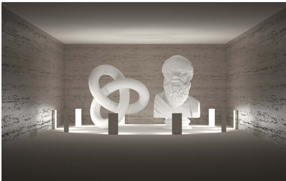
Fig. 3.7 - Emission from the front side of the polygon, diffuse reflection from the back
